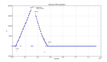
The G1 only provides GPS data up to 60,000' so there is a large gap between samples 2940000 and 3680000 during which the balloon exceeded that altitude.
